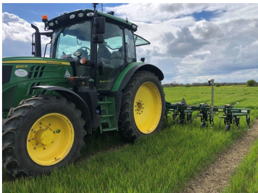
Fig. 3: Inter-Row Hoe working in the Field
