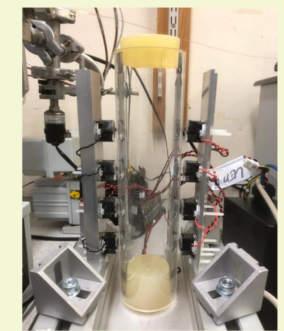
Fig. 6 Prototype of the gas exchange chamber for mass spectrometry.
