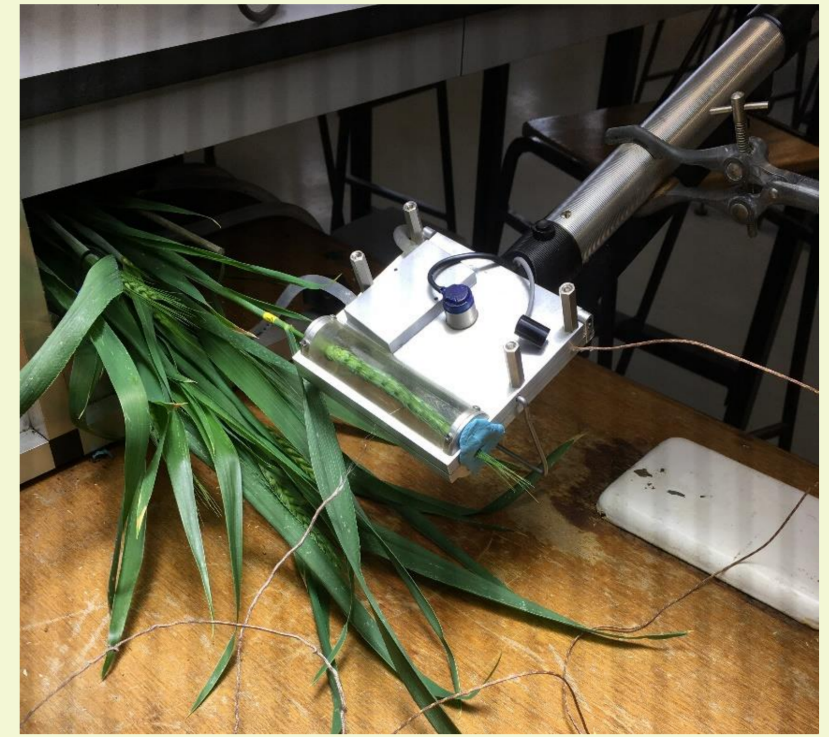
Fig. 4 Custom build gas chamber for wheat ears.
