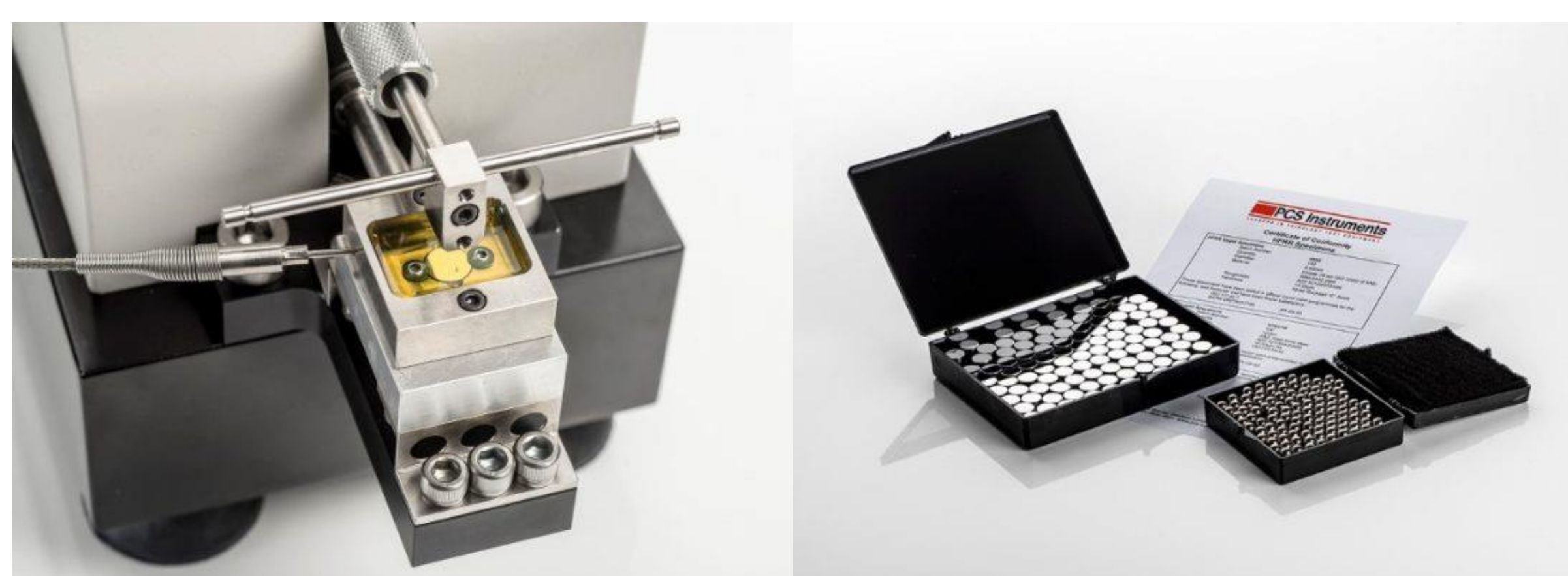
Fig 2: The HFRR (left) and its stainless steel specimens (right) [2].
