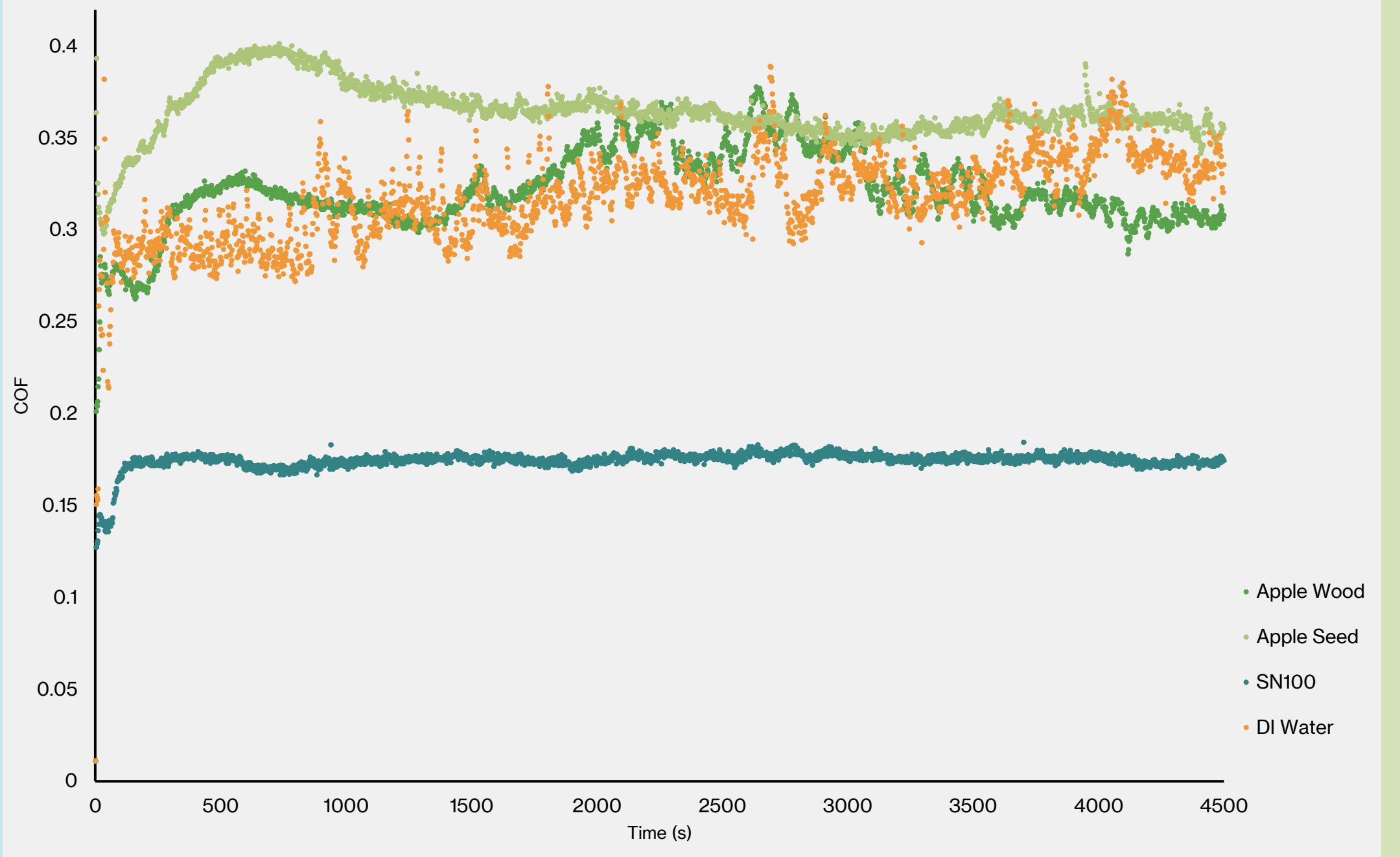
Fig. 3: Mean COF variation throughout HFRR lubricity test.
